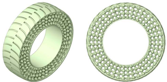
Fig. 6 Conceptual design of a full-scale RPAS tire with an outer diameter of 600 mm, composed of four unit cells in the radial direction.
